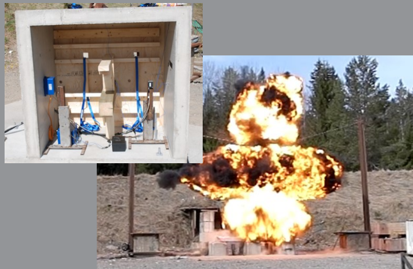
Figure 6. Left: One of the test structures with instrumentation inside. Right: One of the explosives test with the test structure to the left and the blast to the right.
