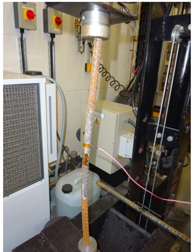
Figure 4. Rebar at a Strain of 2040 \mu \epsilon
